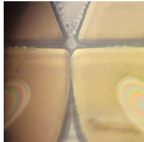
Figure 6.7: Inlet throat of the microfluidic oscillator. The obstruction of the inlet is explained by an over-exposure of the photoresist.
