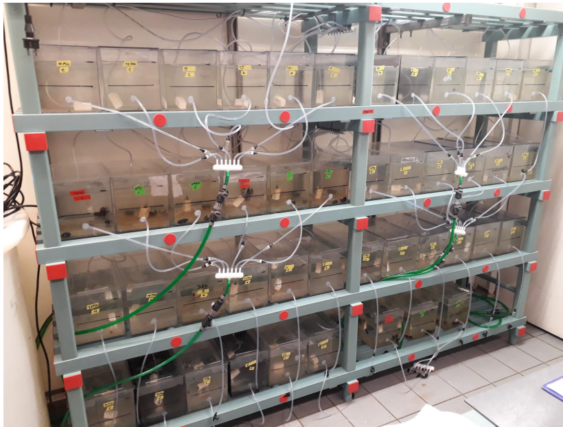
Figure B.6: This figure depicts a part of the climate chamber set up. Here tanks (10 L aquaria, filtered Baltic sea water 0.2 \mu m ) of sea anemones, snails and mussels are shown. Air saturation in experimental tanks was maintained above 80% with air diffusor stones that were placed in each experimental unit. Salinity treatments were positioned randomly. Prior to experiments animals were acclimated to climate chamber conditions.
