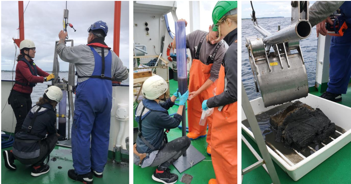
Figure 8 (left): Retrieval of the Frahm lot with seafloor material. (middle): Transferring the sediment core to plugs to secure the specimen. (right): Sediment sampling with Van Veen grab corer.
