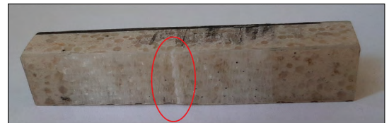
Figure 9. Glass fiber weave and epoxy resin laminated test sample after test, on the surface. Notice the impact formed notch
