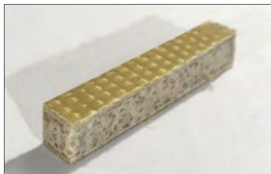
Figure 8. Aramid fiber weave and epoxy resin laminated test sample
