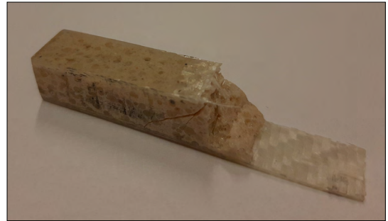
Figure 12. Glass fiber weave and epoxy resin laminated test sample after test
