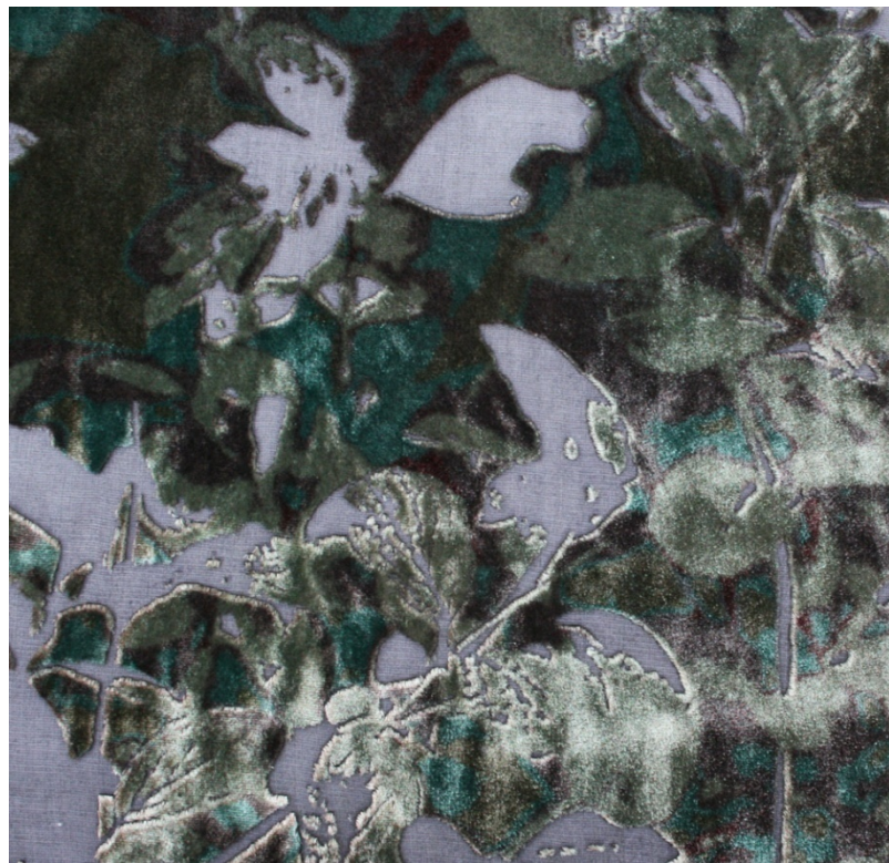
Figure 3.5 (Ryall.H, 2003) Silk Viscose Velvet with Devoré and Reactive Print on Reverse of the Fabric
