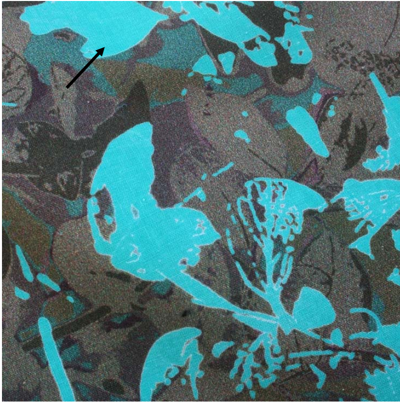
Figure 4.1 (Ryall.H, 2003) Discharge Resist Paste used Prior Ink Jet Printing onto Plain Cotton
