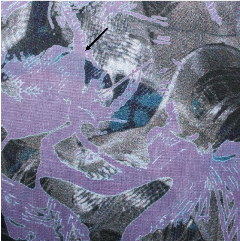
Figure 4.2 (Ryall.H, 2003) Discharge Resist Paste used Prior Ink Jet Printing onto Plain Cotton
