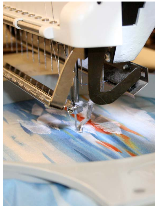
Figure 4.12 (Ryall.H 2009) Amaya® Embroidery Machine, Stitch Pattern onto an Ink Jet Printed Fabric
