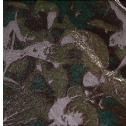
Figure 7: Silk Viscose Velvet with devoré and reactive print on reverse of fabric (21)
