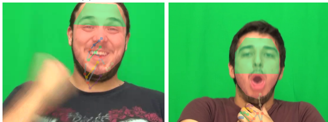
(b) False positive detection caused by a fake hand detection. (c) False positive detection caused by the inaccuracy of the hand landmark detector.
