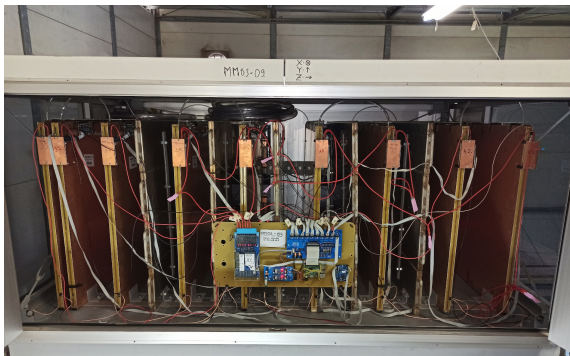
Figure 3. An MMOS with 8 Modified MWPC detectors (green and copper colours are visible) and the lead plates inbetween them, while the corresponding DAQ is mounted to a well-accessible side.
