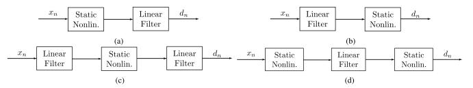
FIGURE 2. Considered system models for (a) the Hammerstein case, (b) the Wiener case, (c) a nonlinearity between two linear filters, and (d) a linear filter between two nonlinearities.
