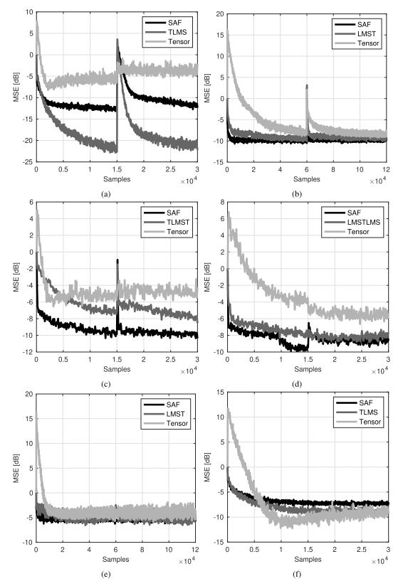
**FIGURE 5.** MSE convergence for all considered algorithms for (a) the Hammerstein case, (b) the Wiener case, (c) a linear filter between two nonlinearities, (d) a nonlinearity between two linear filters, (e) the Wiener case with a nonlinearity depending on past samples, and (f) the Hammerstein case with a nonlinearity containing memory.
