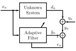
**FIGURE 1.** An overview of the general problem of adaptive system identification.
