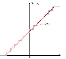
**FIGURE 3.** Discretization of the input signal of the tensor. The input signal  $x_n$  is mapped onto  $N_{\text{Bins}}$  equal intervals to yield the output signal disc  $(x_n)$ . The red line shows discretization with an ideal, infinitely fine grid, and  $\Delta x$  denotes the discretization interval size.
