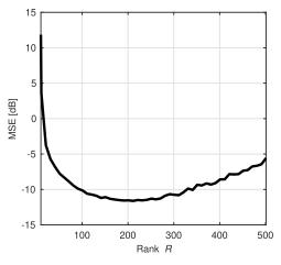
FIGURE 7. The influence of improperly chosen rank R on the performance of the tensor-only architecture in the scenario considered in experiment 6.
