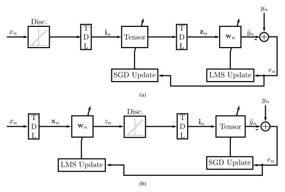
FIGURE 4. The proposed architecture for the (a) tensor-LMS case, and (b) LMS-tensor case, the sandwich approaches are a suitable combination of both architectures. The TDL blocks denote a tapped delay line.
