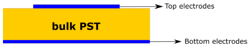
Figure 4.2: Structure of bulk PST for IR Camera. The bulk PST is 0.5 mm thick. The area of the top electrodes seen by the IR Camera is 0.480 \text{ cm}^2
