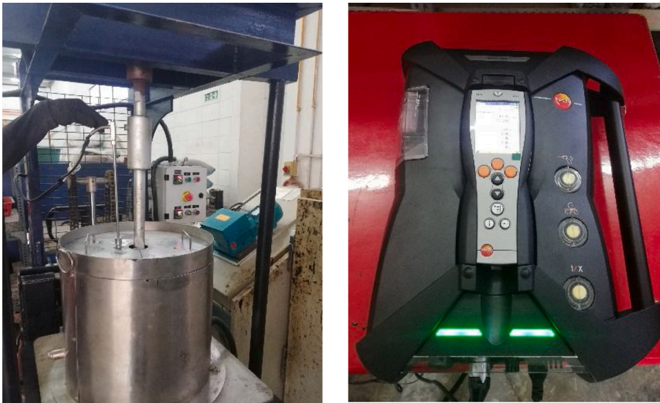
Fig. 1. Asphalt mixer with Testo 350 gas analyser.
