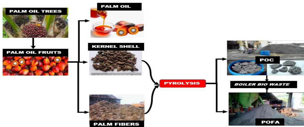
Fig. 2 - Schematic diagram of producing biomass residue in the palm oil mill
