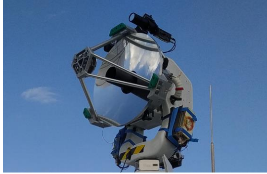
Figure 8. The 60 cm Ritchey-Chrétien-Cassegrain Telescope of DLR-TOGS, with the black 2" Power-Sensor mounted on top next to the primary mirror.
