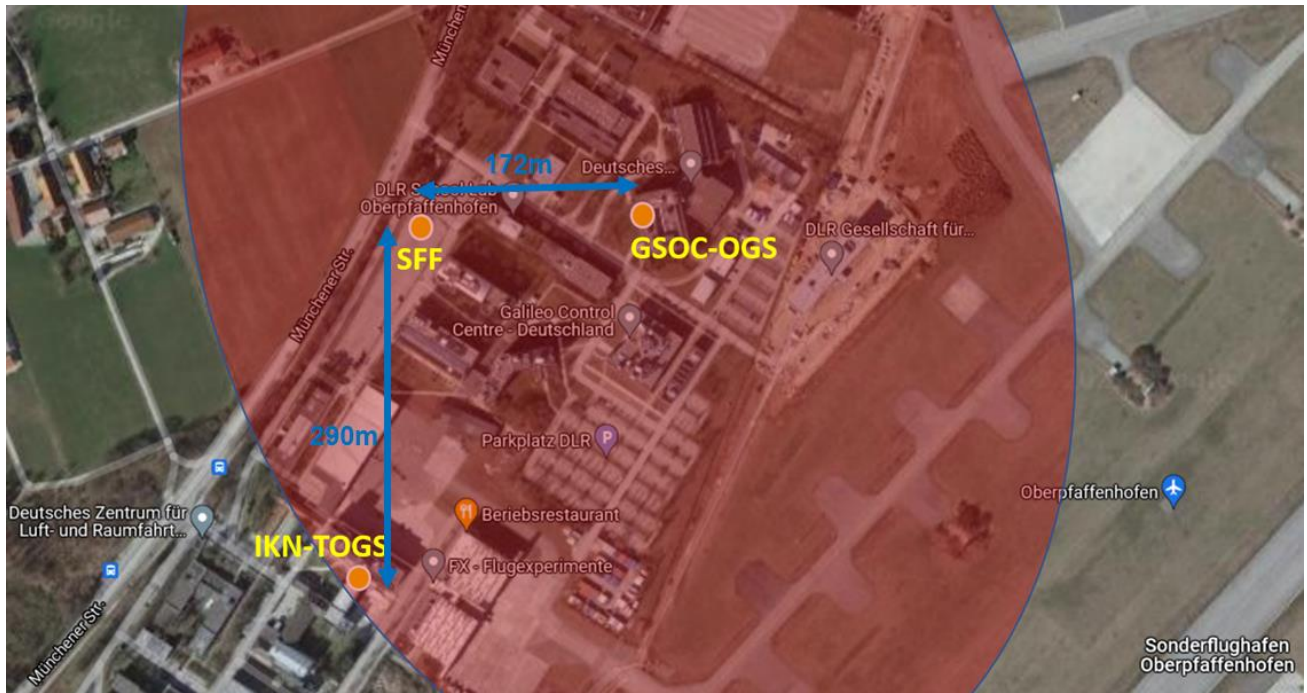
Figure 4. Aerial view of the receiver-site, indicating the locations of the three OGS. North is at top. The red area shows the ideal FWHM beam intensity at ~25° link elevation, centered on the GSOC-OGS. The three OGS-locations approx. resemble a rectangular triangle, with leg distances of: GSOC-SFF ~172m and SFF-IKN ~290m.
