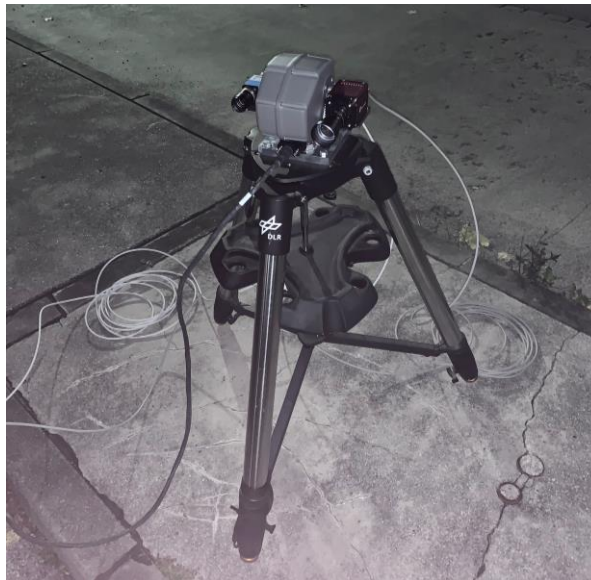
Figure 6. Photograph of the Satellite Flash Finder with an infrared- and a daylight-camera.
