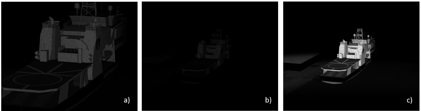
Fig. 3. Simulated sensor images of scenario 1: a) Using the current optics (85 mm lens, f/1.2 ) and optical power (2.5 W). b) Wider FOV (35 mm lens, f/0.8 ) and current optical power (2.5W). c) Wider FOV and 10 times more optical power (25 W).
