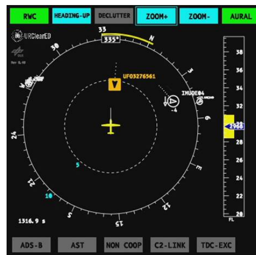
Figure 11. View of the CDTI displaying the surrounding traffic together with the alerting conditions, the horizontal and vertical conflict bands, and the overall status of the DAA RWC system.
