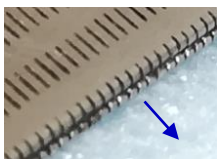
Figure 1: Noise reduction technologies implemented at F16 cruise wing trailing edge for AWB experiment.
