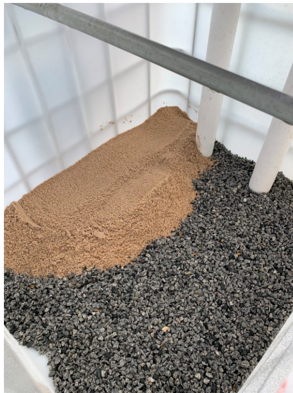
Figure 19: Gingin Quartz on top of 14mm blue gravel drainage layer
