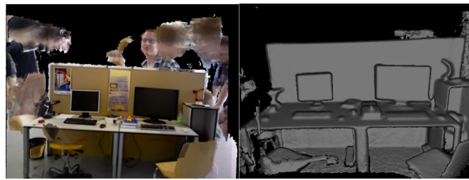
(a) ReFusion (left) vs ACEFusion reconstructions running on the walking_xyz sequence of the TUM RGB-D dataset.
