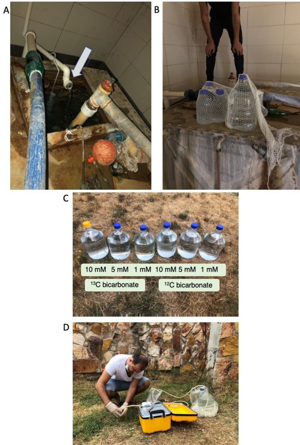
Figure S3: Photographs of the fluid sampling from the 750m deep aquifer and experimental setup, at the private hotel in Bardakçılar village (Biga Peninsula, Turkey). A) Pristine alkaline hydrothermal fluids that were collected, before the geothermal water enters the hotel plumbing system. Arrow shows the fluids that were sampled. The bottles were filled with fluid and incubated at high temperature with the labeled or unlabeled bicarbonate in the square shaped water collector. The bottles were secured in the water collector using fish nets (panel B). C) Incubations with added sodium-bicarbonate. D) Termination of the incubations. A field pump was used to filter the incubated alkaline hydrothermal fluids after the 135 hours of incubation.
