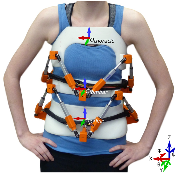
Figure 1.1: Robotic Spine Exoskeleton designed for female adolescents
