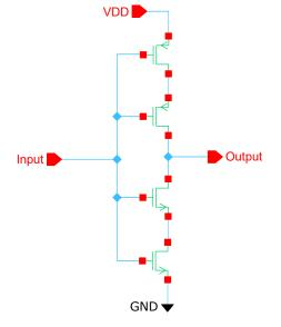
Fig. 8: Schematic of CMOS inverter with stack technique.
