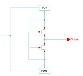
Fig. 5: A generic CMOS circuit with LECTOR technique.
