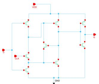
Fig. 3: Schematic of DET-DFF using TSPC logic.
