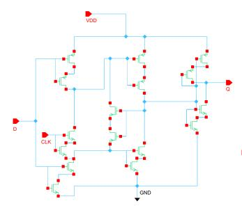
Fig. 11: Proposed circuit of DET-DFF with stack technique incorporated.
