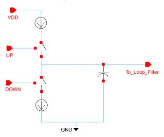
Fig. 2: Schematic of charge pump.
