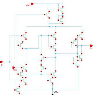
Fig. 13: DET-DFF with AVLS and stack techniques incorporated.
