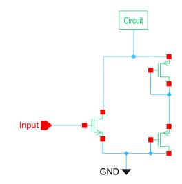
Fig. 7: Basic circuit illustrating AVLG.
