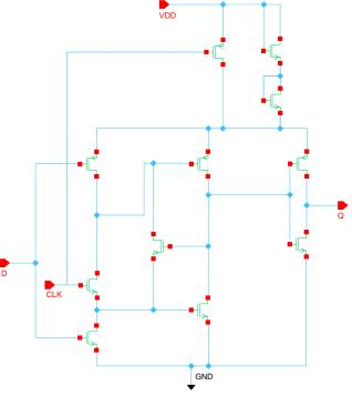
Fig. 10: Proposed circuit of DET-DFF with AVLS incorporated.
