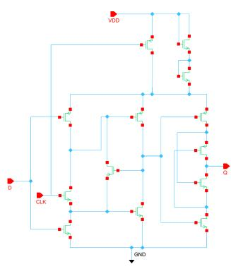
Fig. 12: DET-DFF with AVLS and LECTOR techniques incorporated.
