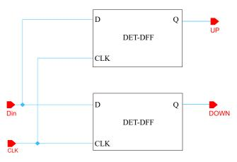
Fig. 4: Schematic of PFD realized using DET-DFF.
