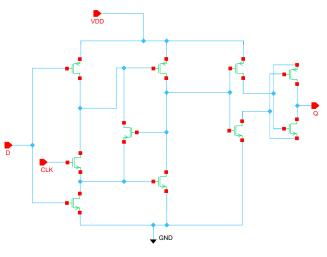
Fig. 9: Proposed circuit of DET-DFF with LECTOR technique.
