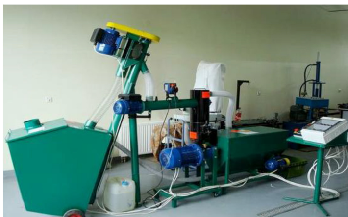
Figure 1. Kovo Novak pellet production line consisting of a hopper, granulation unit, and a cooler for finished pellets.
