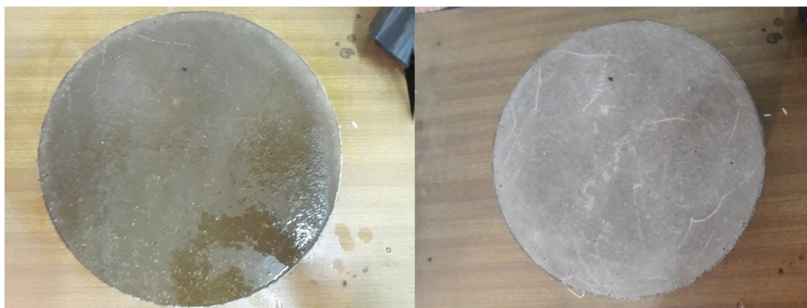
Figure 2. Catalyst containing copper particles shortly after spraying (left) and after the drying process (right).
