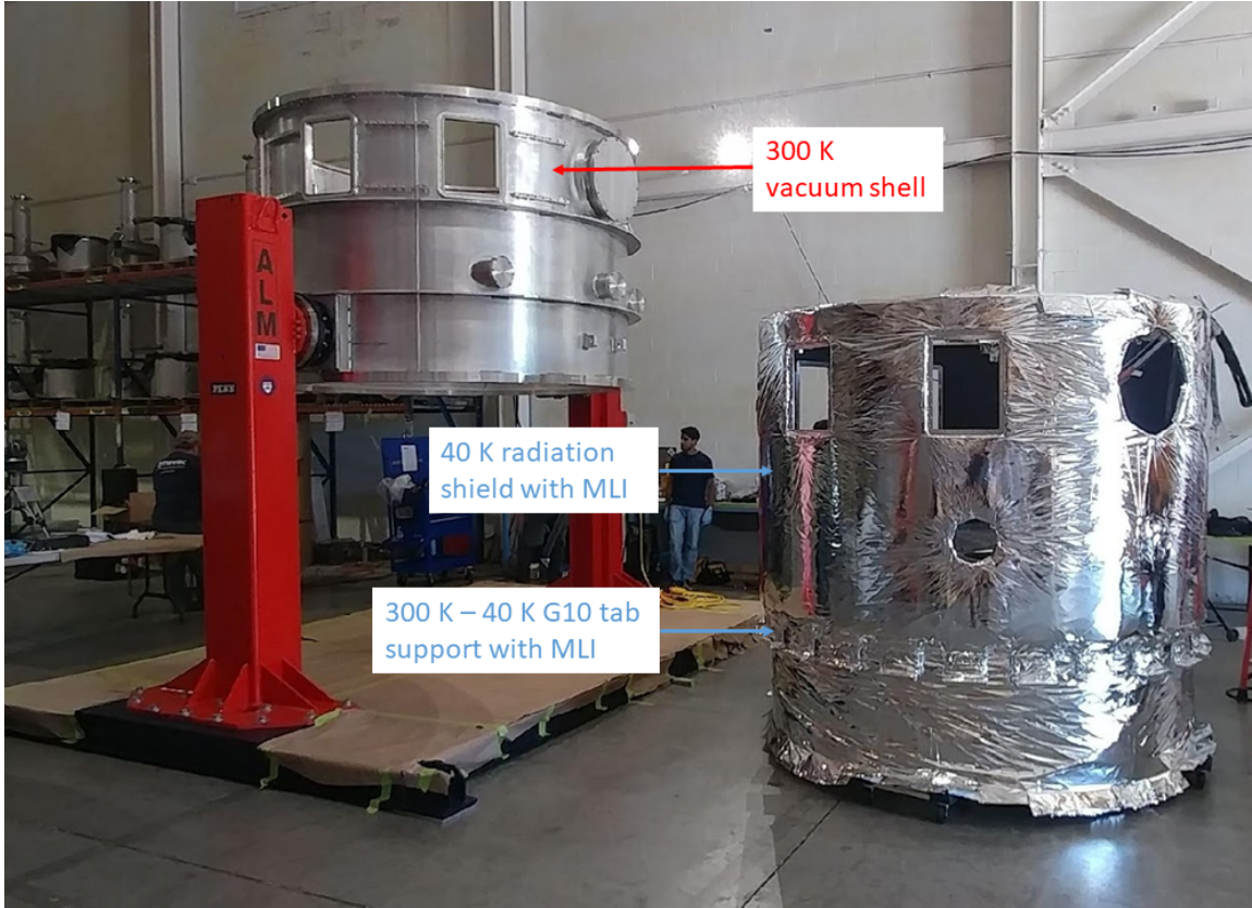
Figure 2.10: This picture shows the 40 K shield assembly sitting on dollies right before getting installed onto the vacuum shell. The 40 K shield is wrapped with 30 layers of MLI. The G-10 tabs attached to the 40 K shield is wrapped with 20 layers of MLI. The black paint inside the 40 K shield is also visible through the radial cutouts.
