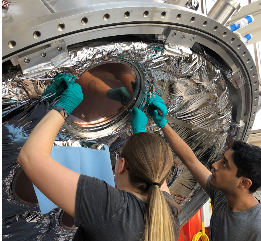
Figure 3.6: In this picture, the cryostat is rotated to face downwards by 45 degrees to provide easy access to the front of the 80 K filter plate. Anna Kofman and Tanay Bhandarkar are installing the 80 K filters onto the 80 K filter plate. This installation has to be performed very carefully to avoid damaging the thin film filter.
