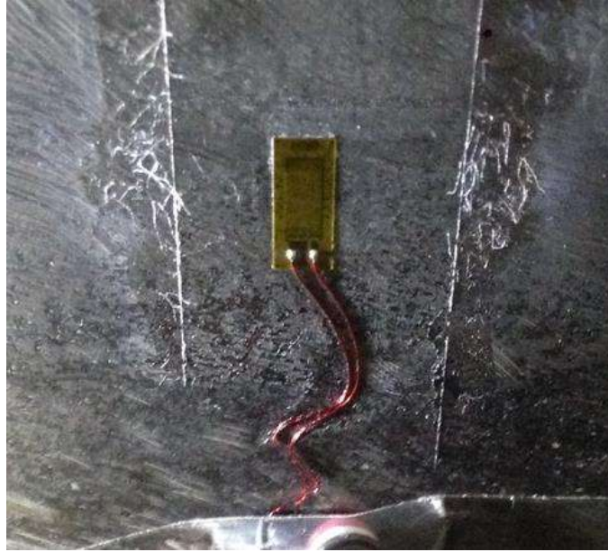
Figure 2.3. Photo of Vishay 350 \Omega quarter-bridge foil strain gage on the web of the rail before protective coating was applied
