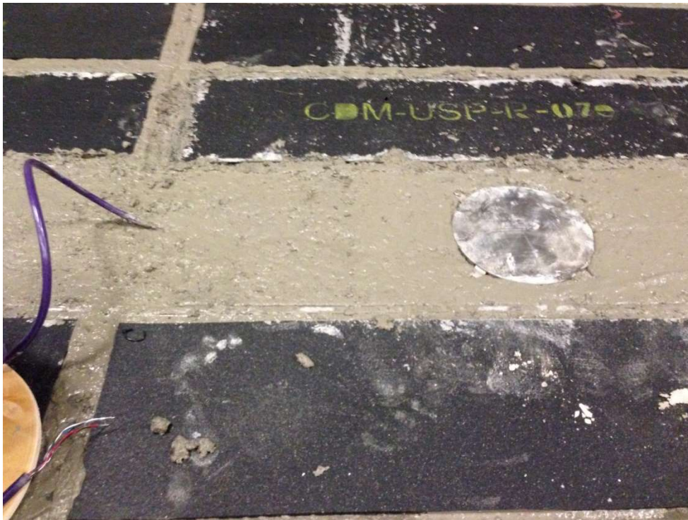
Figure 4.1. Pressure sensor installed in a tie at Rocla Concrete Tie Plant
