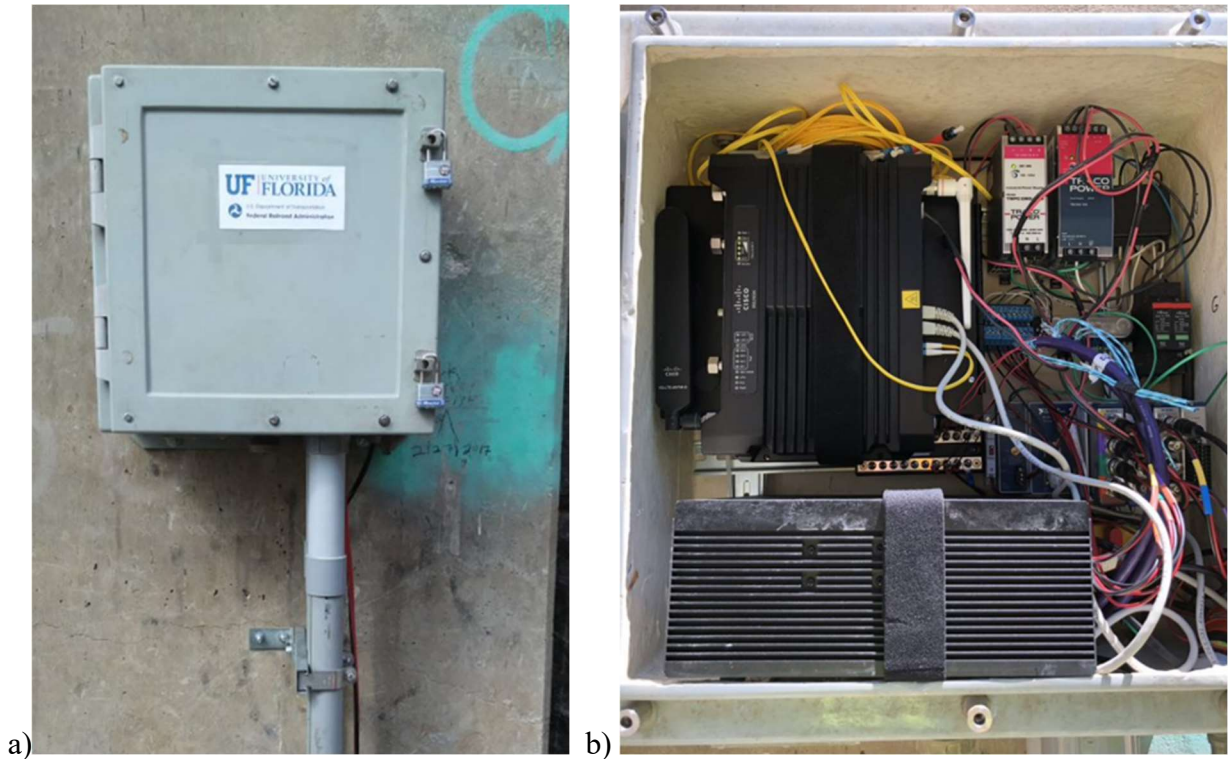
Figure 4.9. Portal DAQ cabinet a) mounted outside of tunnel, and b) inside of Portal DAQ cabinet showing the cellular modem and computer in addition to DAQ components
