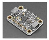
These sensors use a laser range finder to detect distances of up to 1200 cm. The resulting data records the color, the direction, and the distance of an object detected in front of the robot. The robot then takes this data and responds by stopping or turning away from the detected object. See Figures 2.33 and 2.34 for more tests and results.
