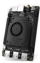
The LattePanda handles all the path planning of the robot. This is because the GPS is directly connected to the computer and the planned route is derived from planning the waypoints. In addition to the RTK GPS and waypoint path planning, the LattePanda also uses an object-detection program through Python TensorFlow.
