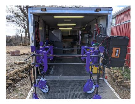
Figure 2.19 shows the designed gussets attached at the remote lab. Each corner of the robot has its own gusset that connects to the according wheel shaft. The result was greatly increased rigidity of the frame, as expected.
