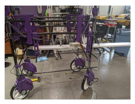
Additionally, as seen in Figure 2.25, there were carbon fiber crossbeams that were originally designed to be just above the fenders. With the addition of the gussets and the braces connecting to the wheel shaft, these lower cross braces would later be removed, reducing weight.
