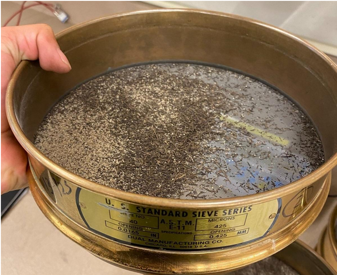
Figure 16: Difficulties in measuring gradation of organic mixed soils
