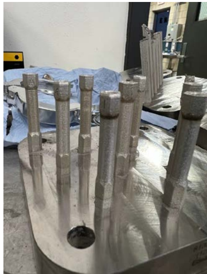
Figure 3.13: Build 4 thin-walled pressure vessels test coupons
