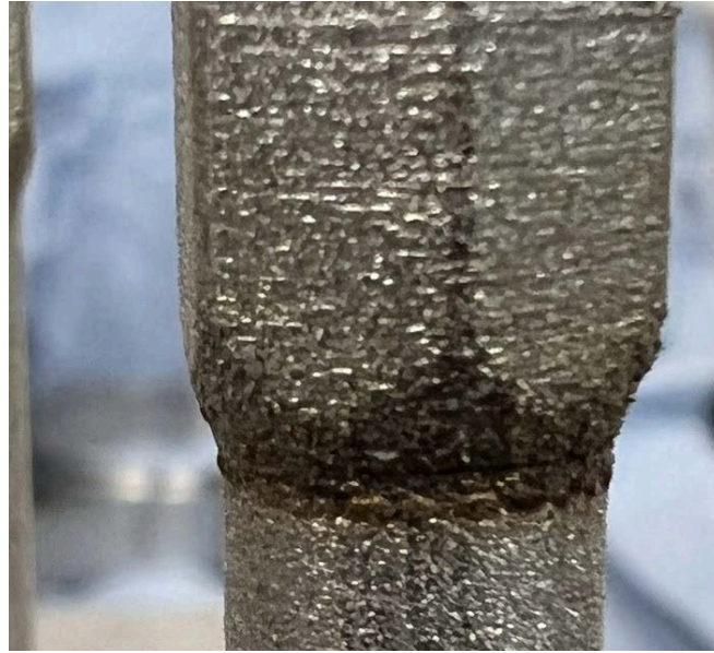
Figure 3.14: Zoomed in image on intersection between hex and main body showing discoloration and potential leak points
