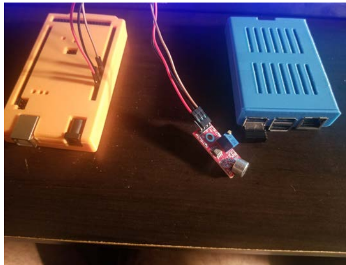
Figure 2.3: Arduino (Left), Devmo sound sensor (Middle), and Raspberry Pi (Right)
