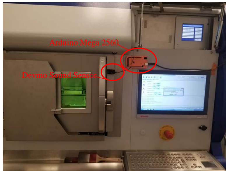
Figure 2.4: Image showing mounting positions of sound sensor and Arduino
