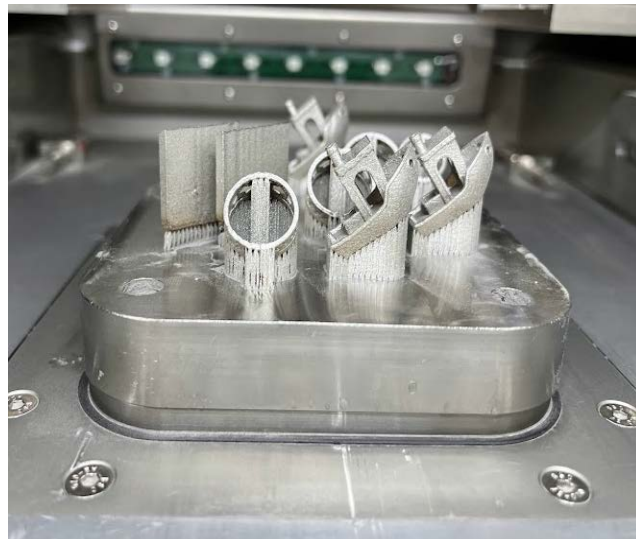
Figure 3.6: Completed Build 3 with parts on build plate (Welding coupons, rings, and benchys)
