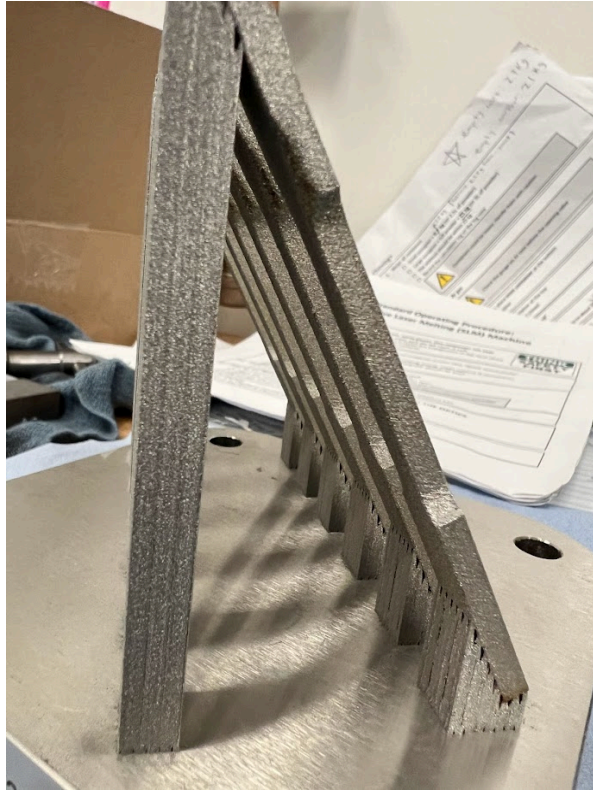
Figure 3.31: Side shot of Build 5 highlighting quality of build with minor discoloration at overhang
