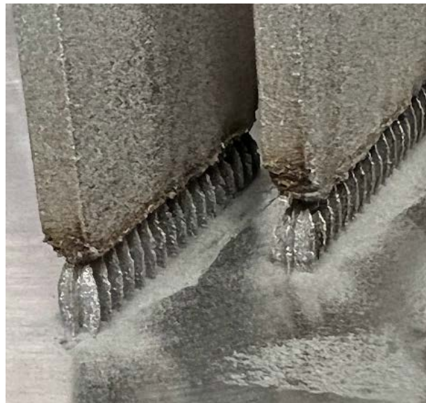
Figure 3.8: Enhanced image of welding coupons, emphasizing the delamination between the part and support structures
