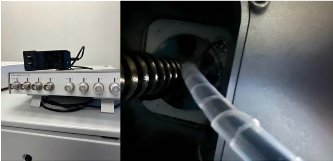
Figure 3.33: Kistler DAQ system (Left), Mounting location under build plate for accelerometers and sound monitor (Right)
