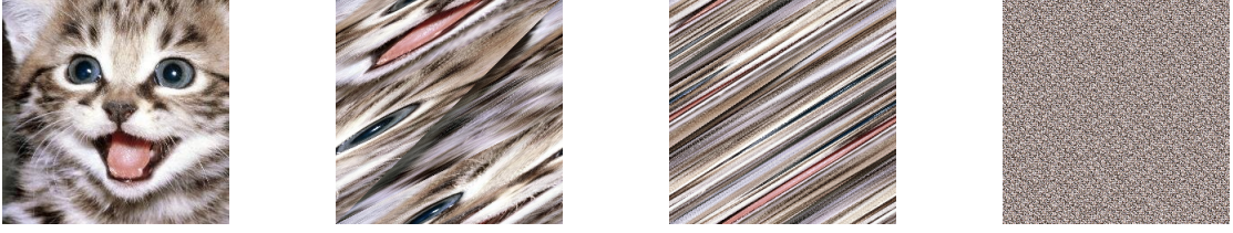
Figure 1.4: Arnold's Cat Map Example. An image of a cat under Arnold's Cat Map, from left to right: base image, 1 iteration, 2 iterations, 128 iterations. It can be shown, on a discrete set such as pixels in an image, that Arnold's Cat Map is periodic [4]. For code, see Appendix A.
