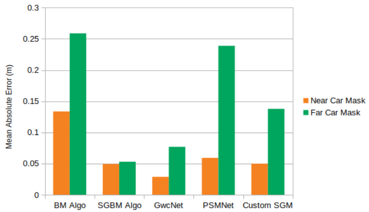
Figure A.6: Comparison of MAE values from depth maps generated by different algorithms in a wide baseline camera configuration of the near and far vehicles
