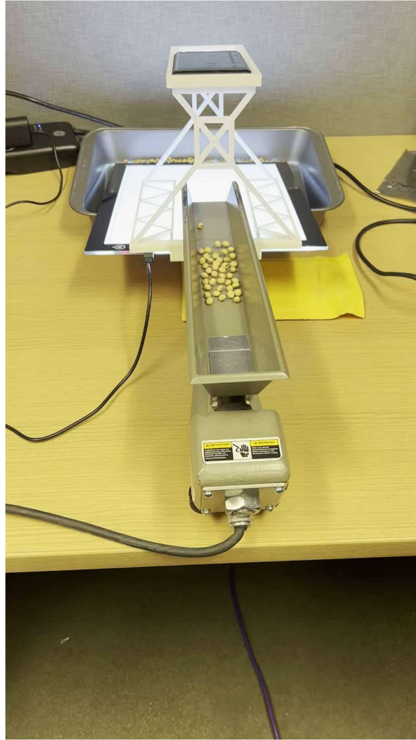
Figure 4.1: Mechanical Hopper Delivering Soy Seed Kernels with a 3-D printed platform at the bottom. The platform at the bottom channels the seed kernels ensures that the seed kernels remain in the field of view of the camera as they roll down the light box. In the absence of the platform, it is observed that seed kernels often drift to the side and fall off the light box prematurely hindering their detection. The mobile phone used for image capture is a Motorola Moto G6 mobile phone whose capture frame rate is 60 fps for HD quality video.
