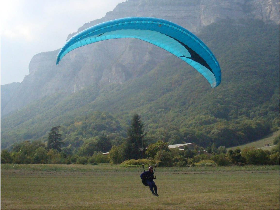
Fig. 5.7: Symmetric brake deflection.
