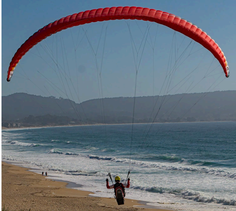
Fig. 8.6: Rear-view of an inflated Hook 3 with symmetric brake deflections
