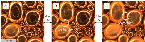
Figure 3: Droplets freezing on the plain surface (Multimedia view). (A) a droplet freezing before bridging to its neighbor. (B) the frozen droplet bridging to its neighbor causing it to freeze. (C) the newly frozen droplet bridging to its neighbor causing it to freeze.
