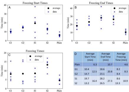
Figure 1: Graphs and table indicating the start, end, and freezing times of the surfaces. (A) The freezing start times of the individual replicates on the different surfaces. (B) The freezing end times of the individual replicates on the different surfaces. (C) The time it takes the surfaces to freeze from start to finish. (D) A table of the averages of the start time, end time, and freezing time.
