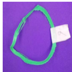
(c) Defect during early stage of printing
