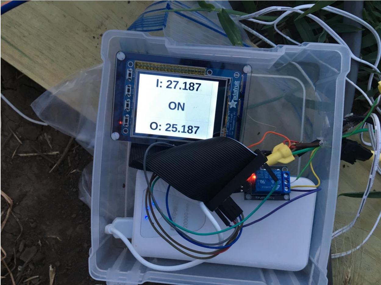
Appendix A Figure - 3 Raspberry Pi touch screen display with interior and exterior temperature.
