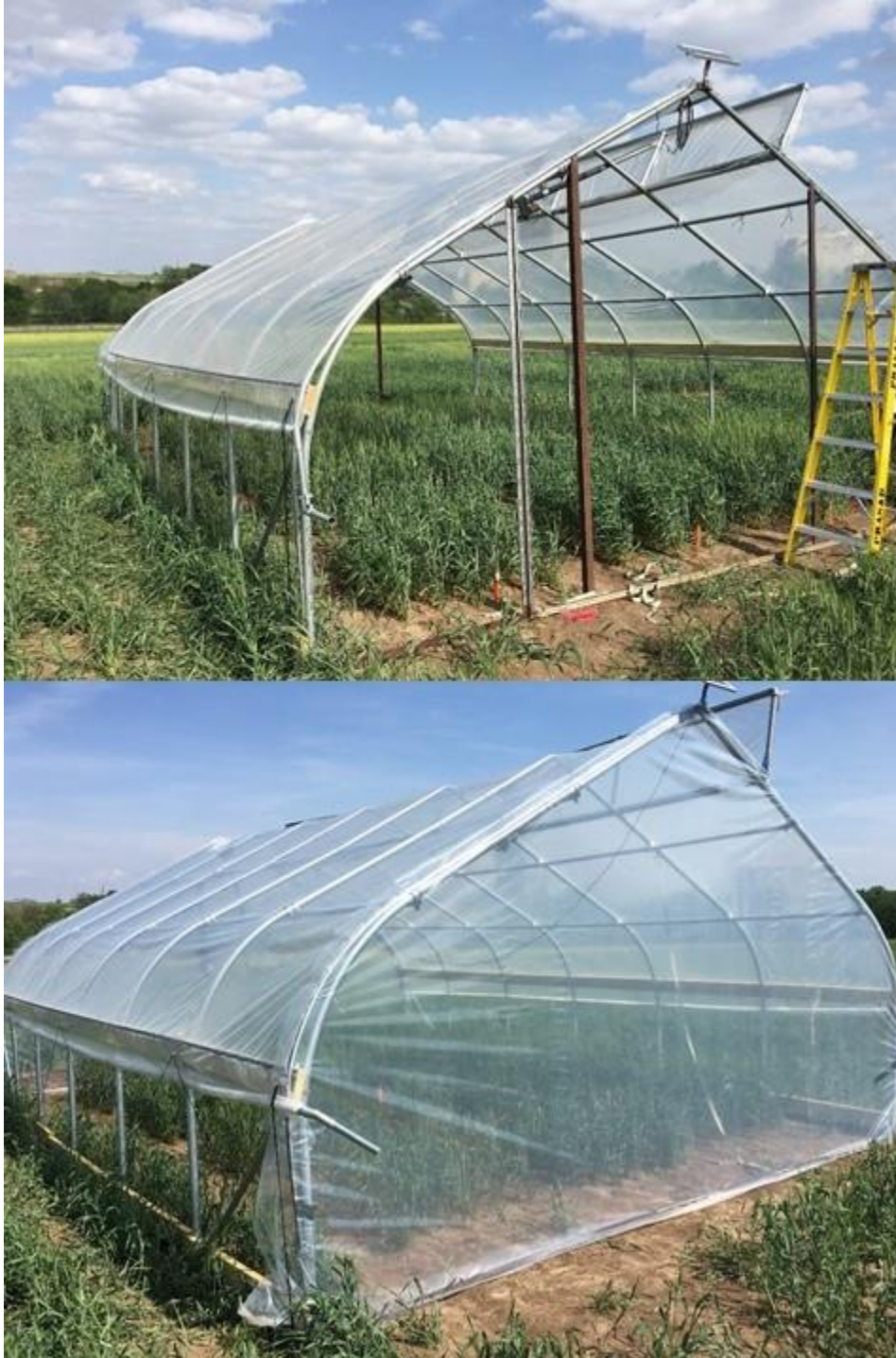
Appendix A Figure - 1 Heat tent before and after end wall plastic application
