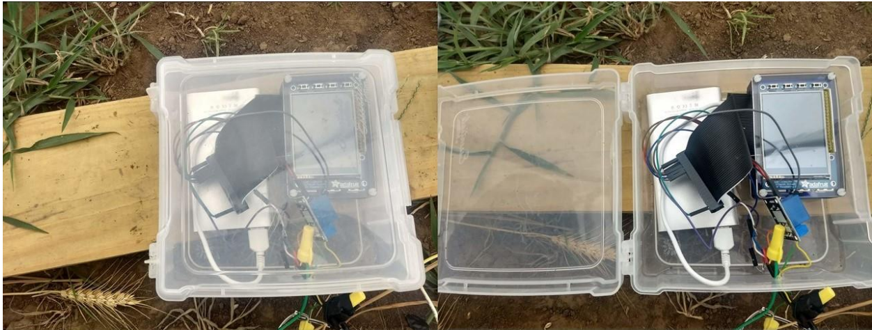
Figure 2-3 Waterproof enclosure for Raspberry Pi and electric system
