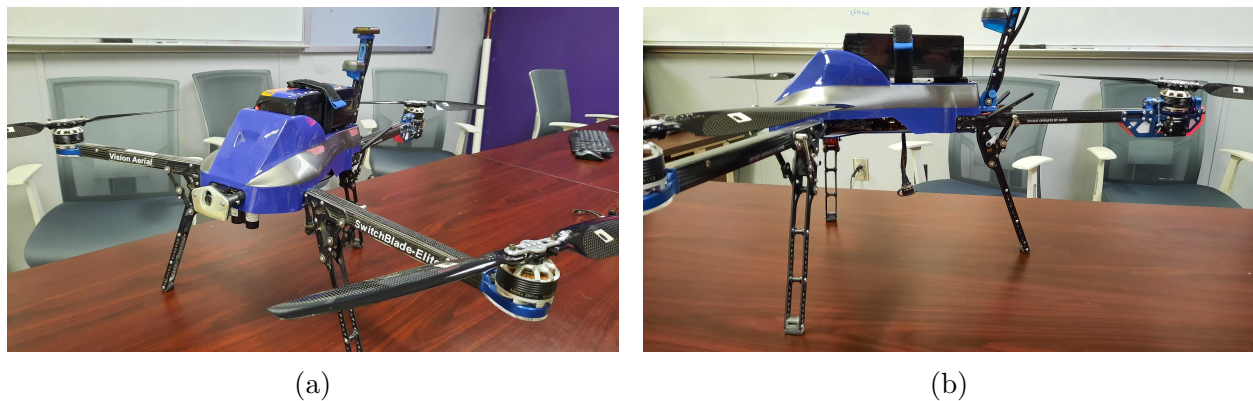
Figure 3.4: Standard flight configuration of the Vision Aerial SwitchBlade-Elite UAV shown in (a) an angled view with downward-facing LiDAR and (b) side view. A >1 -kg payload can be mounted to the bottom of the unit.
