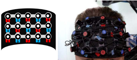
Fig. 2. Channels montage and representation of the whole setup device –in our case, the hardware was placed behind the passenger seat.
