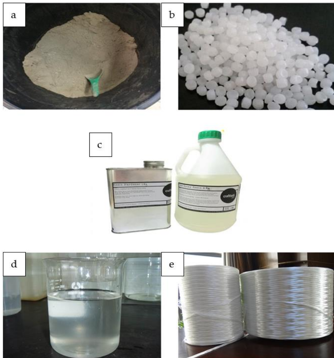
Figure 1. Starting materials. (a) High calcium pozzolanic, (b) sodium hydroxide pellet, (c) epoxy resin (DGEBA) and epoxy hardener (IPDA), (d) sodium silicate liquid, and (e) fiber glass type E.
