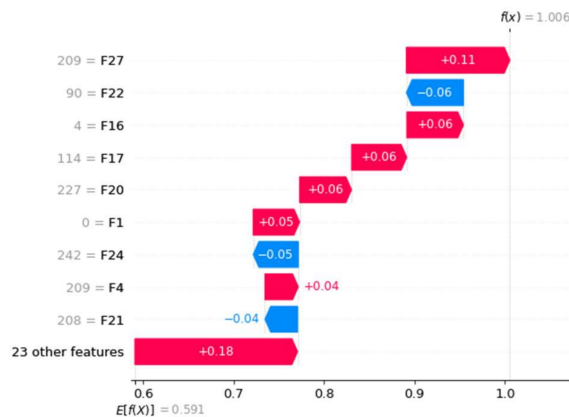
Figure 13. Waterfall plot shows how SHAP values of each feature affect model output compared to the data distribution.
