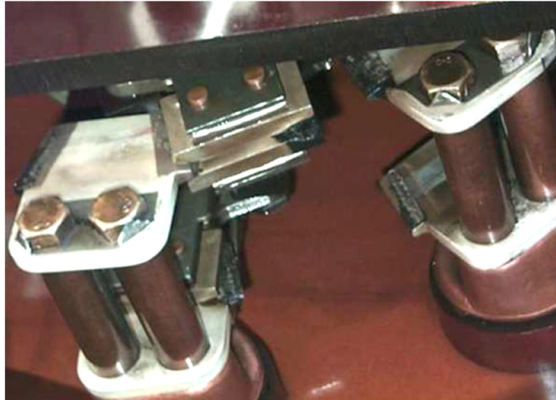
Figure 6. Burned contacts on stationary and movable contacts [14].
