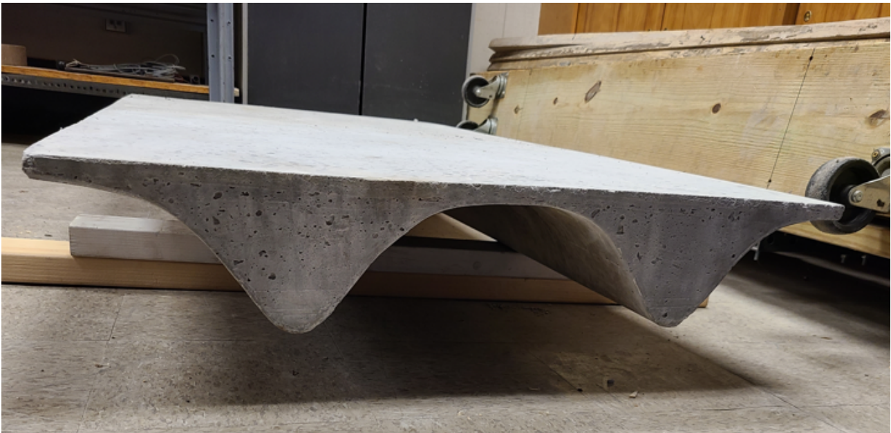
Fig 2 Shaped concrete slab specimen.
