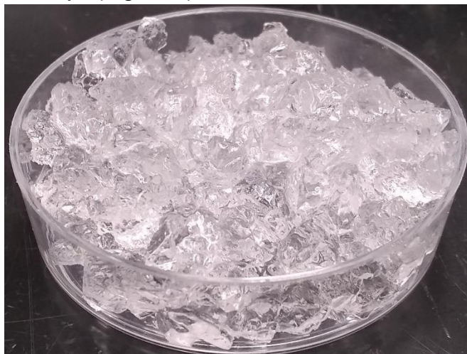
Figure 2. (R)-linalool conditioned in 100-fold saturated polyacrylamide.
