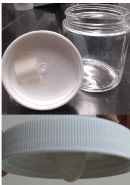
Figure 1. Thrips fumigation chamber with hydrogel “pouch”.
