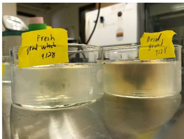
Figure 21. An example of the soil analog experiment, where 200mg of strawberry guava leaf (shown here as fresh or freeze dried) was ground with liquid nitrogen then inserted into the center of a dish (9 x 4.5 cm) containing 200mL of cooled autoclaved 0.4% agar culture medium. A central cylinder core had been excavated (2cm diameter x 1.75cm deep), into which the material was inserted and covered with remaining agar culture medium cooled to 40°C. Lettuce ( Lactuca sativa L.) seeds, as the test species, were placed on the agar culture medium in three concentric circles at increasing 10mm intervals from the core.
