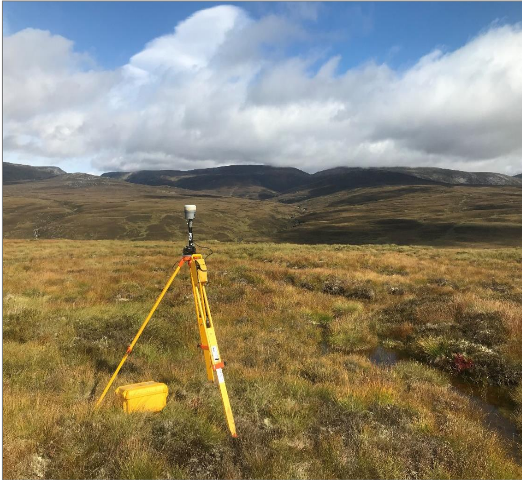
Figure 4.1.2. Trimble R10 GNSS BASE.
