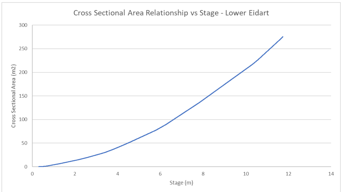
Figure 5.3.2 The Relationship Between Stage and Area for Lower Eidart and Upper Feshie.
