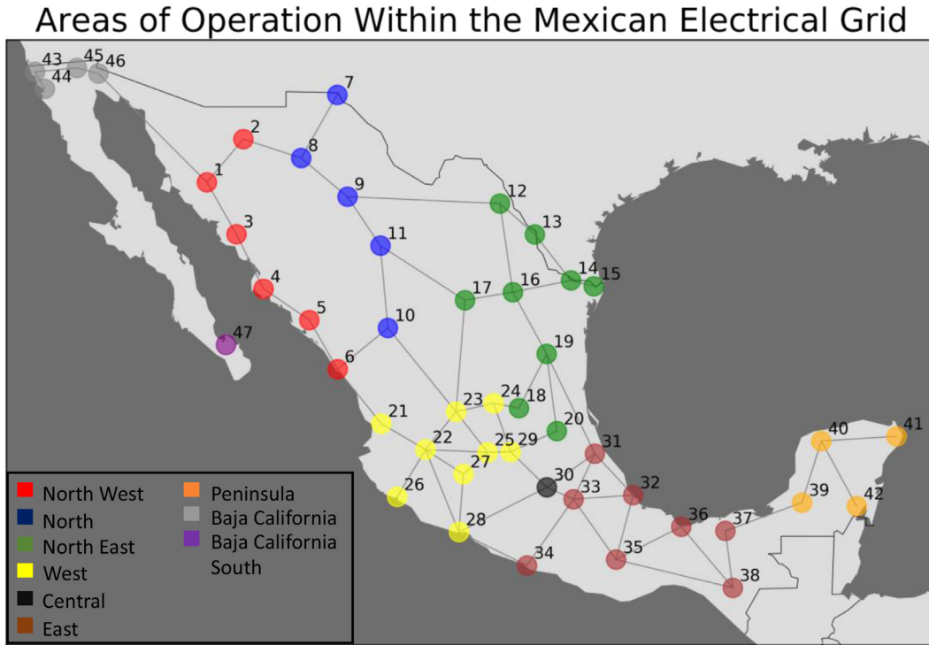
Fig. 8. Mexican electrical grid in PEGyT model. Small numbers at each node indicate demand or production points within the system, color indicates area of operation.
