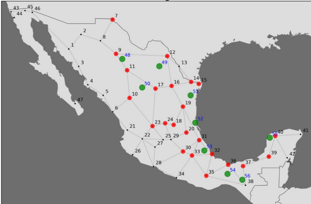
Fig. 10. Mexican electrical grid and storage sites. Black nodes indicate potential generation or demand nodes within the electricity grid. Red nodes indicate nodes within the electricity grid where CCS generation plants can be deployed. Green nodes indicate potential CO_2 storage sites. gray lines indicate connections within the transmission system.
