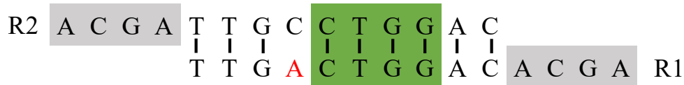
Figure 2.2: An example of adapter removal. This read pair has forward R1 TTGACTGGACACGA and backward R2 GTCCAGGCAATCGT (reverse-complement ACGATTGCCTGGAC denoted as R2^T ). Suffix of R2^T can be matched to the prefix of R1 with an overlap size of 10 including 1 mismatch, indicating fragment length is shorter than read length. Therefore, Chromap removes ACGA from R1 and R2^T (TCGT in R2) as parts of the adapter sequences.
