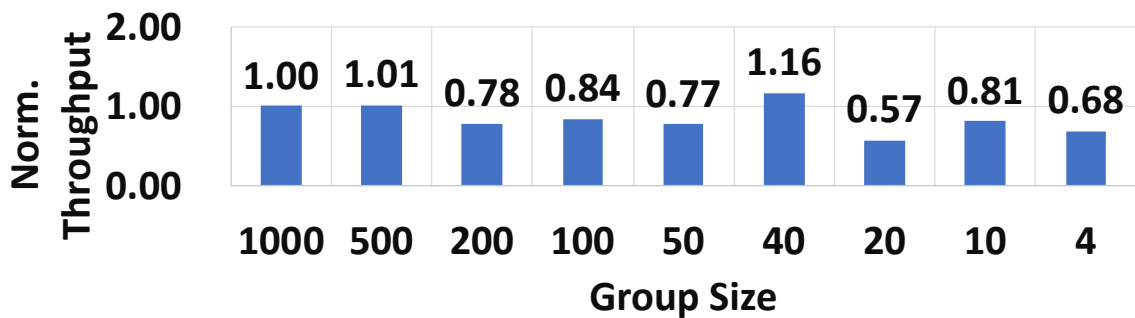
Fig. 7.13: The reached performance of MAGMA given the same task and setting (Mix, S2, BW=16) with different group sizes. Throughput values are normalized by the value of group size=1000,
