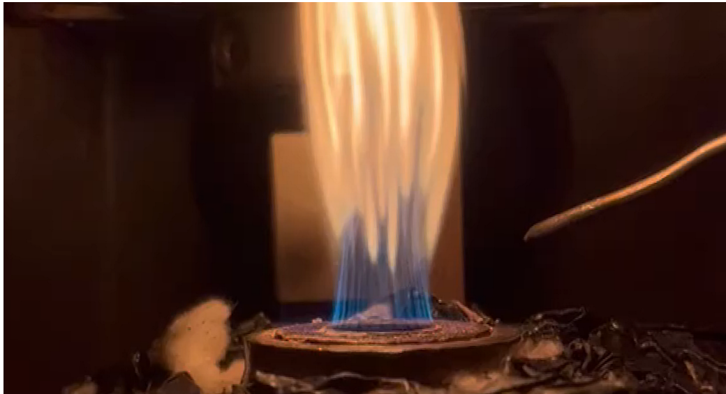
Figure 1.1: Soot formation in a laminar jet-A air flame
