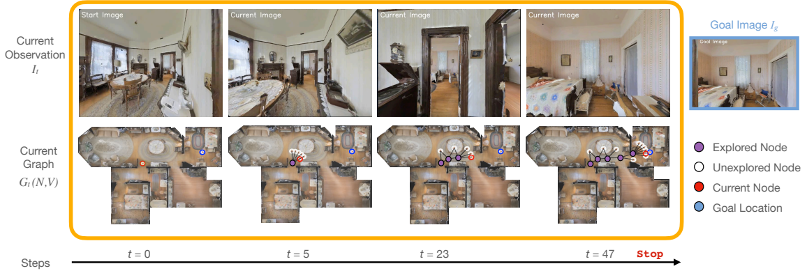
Figure 4.6: Example of an Image-Goal Navigation episode on MP3D. Shows the agent’s observations and internal topological graph at different time steps.
