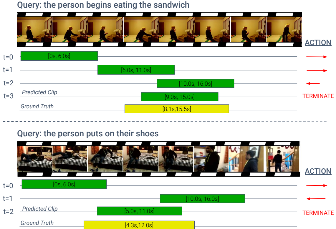
Figure 3.3: Qualitative results of TripNet-GA on the Charades-STA dataset. The green boxes represent the bounding window of the state at time t and the yellow box represents the ground truth bounding window. The first video is 33 seconds long (792 frames) and the second video is 20 seconds long (480 frames). In both examples the agent navigates both backwards and forwards in the video. In the first example, TripNet sees 408 of the frames of the video, which is 51% of the video. In the second example TripNet sees 384 frames of the video, which is 80% of the frames.
