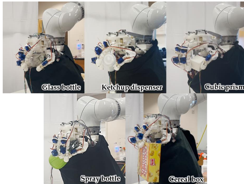
Figure 47: Grasps formed for each of the five objects: (Top left) glass bottle, (Top middle) ketchup dispenser, (Top right) cubic prism, (Bottom left) spray bottle, (Bottom right) cereal box.
