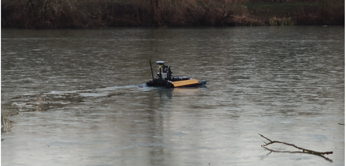
Figure 5.21: Our agent controlling the USV on a frozen lake. The agent follows the shore and maintains a target velocity while breaking 4mm thick ice.
