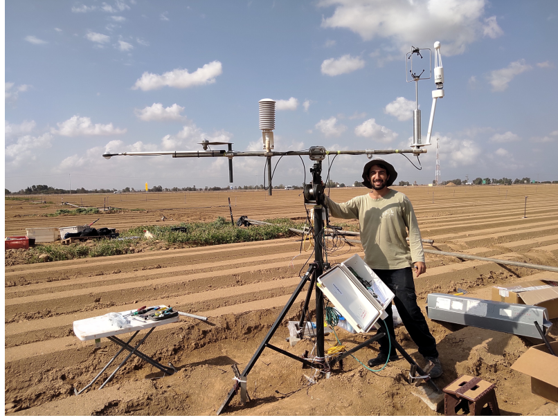
Figure 3.4: An eddy covariance tower in a field. Coworker for scale.
