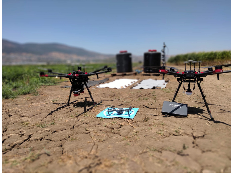
Figure 3.3: The UAVs used when collecting aerial images in the fields.
