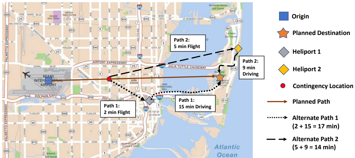
(a) Heliport 2 is selected with the least sum of flight and passenger recovery time in the first scenario of original destination disruption
